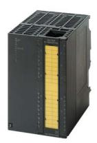
SIMATIC S7, Digital output SM 326, F-DO 8x24 V DC/2A PM fail-safe digital output Switching to P-M potential up to Category 4 (EN 954-1)/ SIL3 (IEC61508)/PLE (ISO13849), 1x 40-pole
