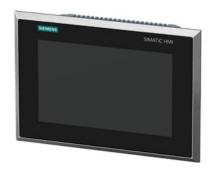
SIMATIC HMI TP900 Comfort INOX Stainless steel front, Glass pane, capacitive touch, Degree of protection front IP69K, 9" widescreen TFT display, PROFINET interface, MPI/PROFIBUS DP interface, 12 MB configuration memory, Windows CE 6.0, (Microsoft Support included Security updates discontinued) configurable from WinCC Comfort V15
