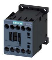
power contactor, AC-3e/AC-3, 12 A, 5.5 kW / 400 V, 1 NO, 24 V DC 3-pole, frame size S00 screw terminal
