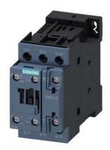
power contactor, AC-3e/AC-3, 12 A, 5.5 kW / 400 V, 3-pole, 24 V DC, auxiliary contacts: 1 NO + 1 NC, screw terminal
