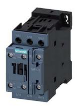
power contactor, AC-3e/AC-3, 25 A, 11 kW / 400 V, 3-pole, 24 V DC, auxiliary contacts: 1 NO + 1 NC, screw terminal
