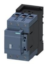
capacitor contactor, AC-6b 100 kVAr, / 400 V, 3-pole, 24 V AC, 50 Hz, auxiliary contacts: 1 NO + 1 NC, screw terminal, size: S3
