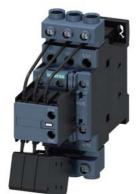
capacitor contactor, AC-6b 33 kVAr, / 400 V, 3-pole, 24 V AC, 50 Hz, auxiliary contacts: 1 NO + 2 NC, screw terminal, size: S0
