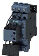
capacitor contactor, AC-6b 33 kVAr, / 400 V, 3-pole, 230 V AC, 50 Hz, auxiliary contacts: 1 NO + 2 NC, screw terminal, size: S0
