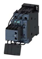
capacitor contactor, AC-6b 16.7 kVAr, / 400 V, 3-pole, 24 V DC, auxiliary contacts: 1 NO + 2 NC, screw terminal, size: S0  $\,$
