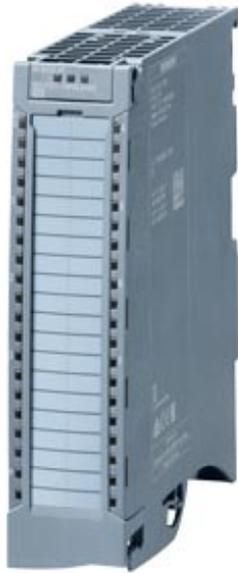
SIMATIC S7-1500 analog input module AI 8xU/I HF, up to 24 bit resolution, accuracy 0.1%, 8 channels in groups of 1; common mode voltage: 30 V AC/60 V DC, Diagnostics; Hardware interrupts Measured values scalable, measuring range adjustment, Calibrate in RUN; Delivery including infeed element, shield bracket and shield terminal: Front connector (screw terminals or push-in) to be ordered separately
