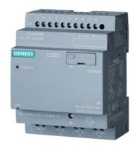
\*\*\* spare part \*\*\* LOGO! 12/24RCEO, logic module, PS/I/O: 12/24VDC/relay, 8 DI (4 AI)/4 DO, without display, memory 400 blocks, modularly expandable, Ethernet, integr. web server, data log, user-defined web pages, standard microSD card for LOGO! Soft Comfort V8 or higher, older projects executable
