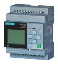
\*\*\*spare part\*\*\* SIPLUS LOGO! 24CE based on 6ED1052-1CC08-0BA0 with conformal coating, -25...+60 °C, start up -20 °C, logic module, display power supply / I/O: 24 V/24 V/24 V trans., 8 DI (4 AI)/4 DQ, memory 400 blocks, modularly expandable, Ethernet integrated web server, data log, user-defined web pages, standard microSD card for LOGO! Soft Comfort V8 or higher, older projects executable
