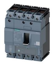
circuit breaker 3VA1 IEC frame 160 breaking capacity class S Icu=36kA @ 415V 4-pole, line protection TM220, ATFM, In=20A overload protection Ir=14A...20A short-circuit protection Ii=16 x In N conductor unprotected clamp connection
