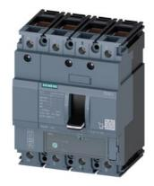
circuit breaker 3VA1 IEC frame 160 breaking capacity class S Icu=36kA @ 415V 4-pole, line protection TM220, ATFM, In=80A overload protection Ir=56A...80A short-circuit protection Ii=10 x In N conductor unprotected clamp connection
